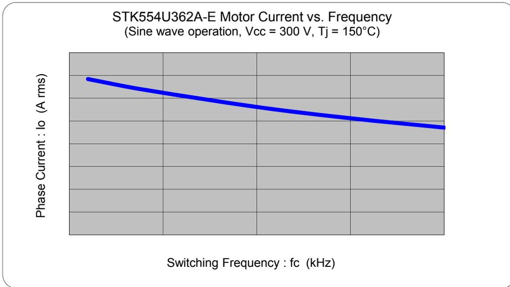
Fig.11 Maximum sinusoidal phase current as function of switching frequency at  $T_c = 100^\circ\text{C}$ ,  $V_{CC} = 300\text{ V}$
