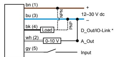
\* Push-Pull output. User-configurable PNP/NPN setting.
