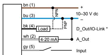
\* Push-Pull output. User-configurable PNP/NPN setting.
