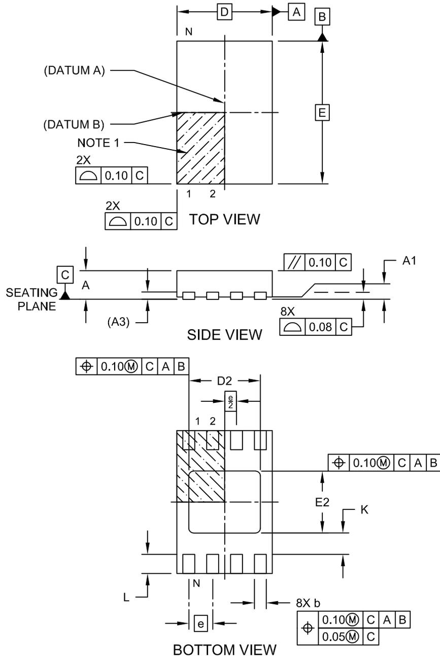
**8-Lead Ultra Thin Plastic Dual Flat, No Lead Package (Q4B) - 2x3 mm Body [UDFN]
