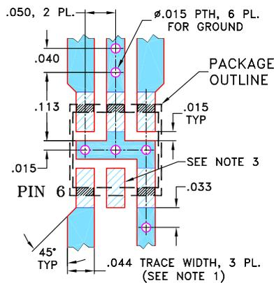
1. TRACE WIDTH IS SHOWN FOR ROGERS R04350B WITH DIELECTRIC THICKNESS .020" ± .0015"; COPPER: 1/2 OZ. ON EACH SIDE. FOR OTHER MATERIALS TRACE WIDTH MAY NEED TO BE MODIFIED.
