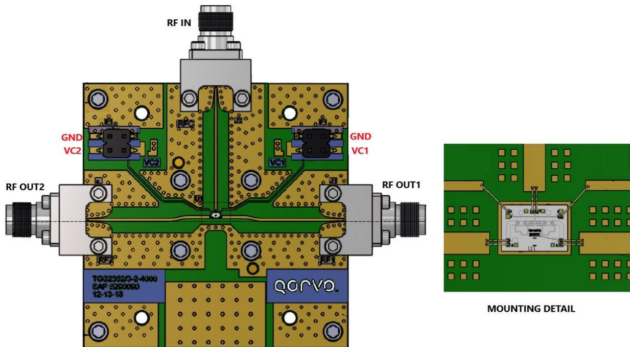
RF Layer is 0.010" thick Rogers Corp. RO4350B,  $\epsilon_r = 3.48$ . Metal layers are 0.5 oz. copper. The microstrip line at the connector interface is optimized for the Southwest Microwave end launch connector 1092-02A-5.
