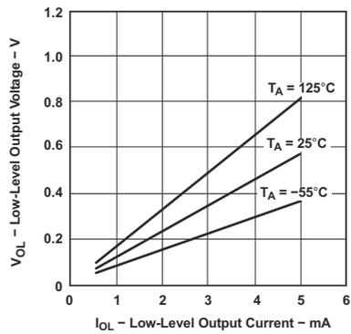
Figure 6-3.  $V_{OL}$  vs  $I_{OL}$
