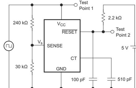
Figure 6-8.  $V_{CC}$  vs Output Test Circuit 1
