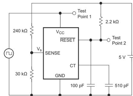
Figure 6-10.  $V_{CC}$  vs Output Test Circuit 2
