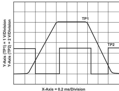
Figure 6-7.  $V_{CC}$  vs Output Waveform 1 - See Figure 6-8
