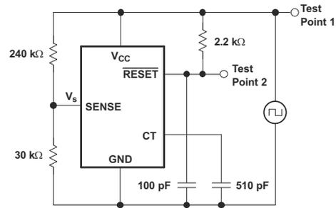
Figure 6-12.  $V_{CC}$  vs Output Test Circuit 3
