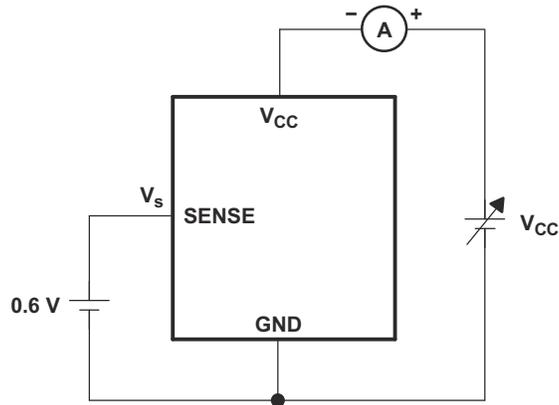
Figure 7-1. V<sub>CC</sub> vs I<sub>CC</sub> Measurement Circuit
