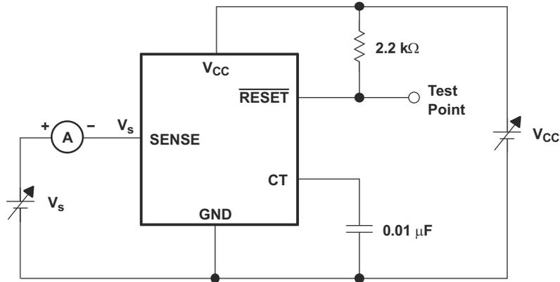
**Figure 7-4.  $V_s$  and  $I_s$  Characteristics Measurement Circuit**
