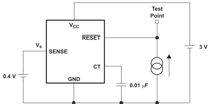
Figure 7-3. I<sub>OL</sub> vs V<sub>OL</sub> Measurement Circuit
