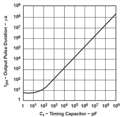
Figure 6-6. Output Pulse Duration vs Timing Capacitor
