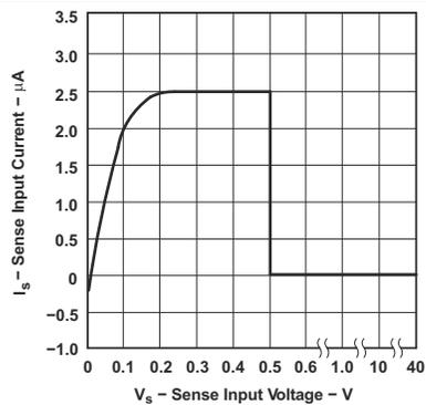
Figure 6-5. Sense Input Current vs Sense Input Voltage
