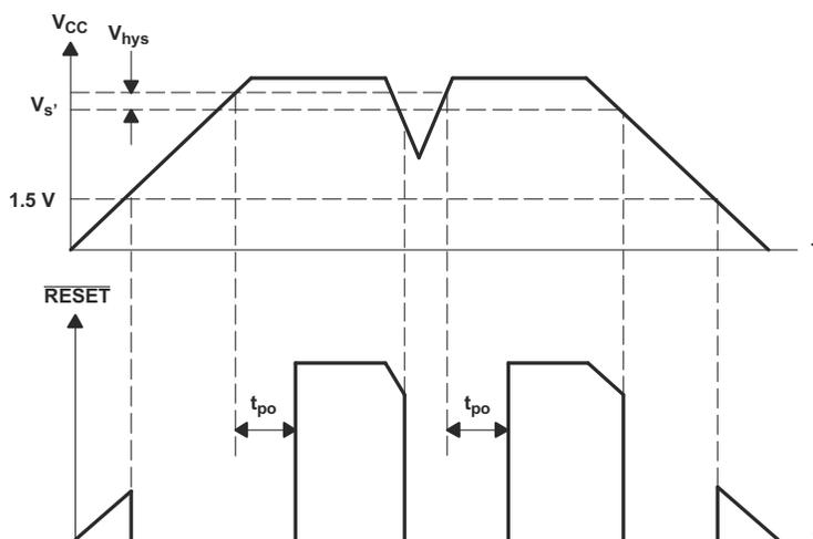
The desired sense voltage ( $V_s'$ ) is different from the SENSE input voltage ( $V_s$ ).  $V_s'$  is typically 500 mV for triggering.
