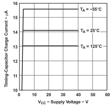
Figure 6-2. Timing Capacitor Charge Current vs Supply Voltage
