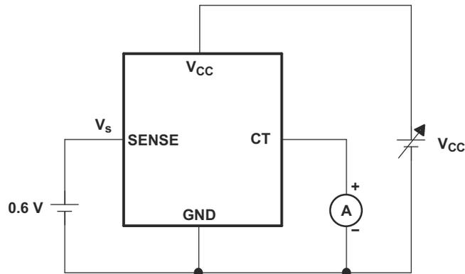
Figure 7-2. V<sub>CC</sub> vs I<sub>CT</sub> Measurement Circuit
