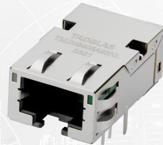
Featuring a popular footprint and compatible package to industry RJ45 Integrated Connectors standards, the Taoglas TMJM9405A93NL is an RJ45 Integrated Connector 10G Base-T Single Port Tab Down with shielded EMI Finger and low-profile body design that offers extra space.
