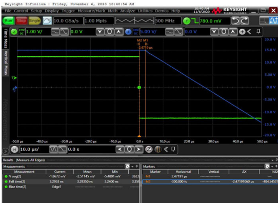
Figure 13. Positive Overload Recovery Voltage: 5 V/div for Output, Time: 10 \mu s/div G = 10 , V_{REF} = GND ; V_{IN} = 5 V_{PP}
