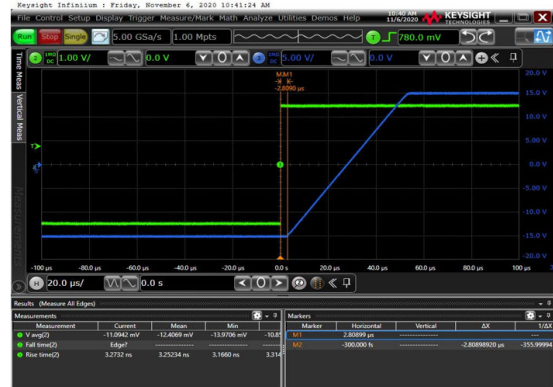
Figure 14. Negative Overload Recovery Voltage: 5 V/div for Output, Time: 10 \mu s/div G = 10 , V_{REF} = GND ; V_{IN} = 5 V_{PP}
