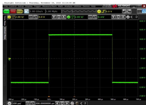
Voltage: 5 V/div, Time: 100 \mu s/div R_L = 2 k\Omega , C_L = 100 pF , G = 1
