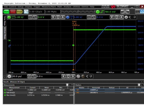
Voltage: 5 V/div for output, Time: 10 \mu s/div G = 10 , V_{REF} = GND ; V_{IN} = 5 V_{PP}
