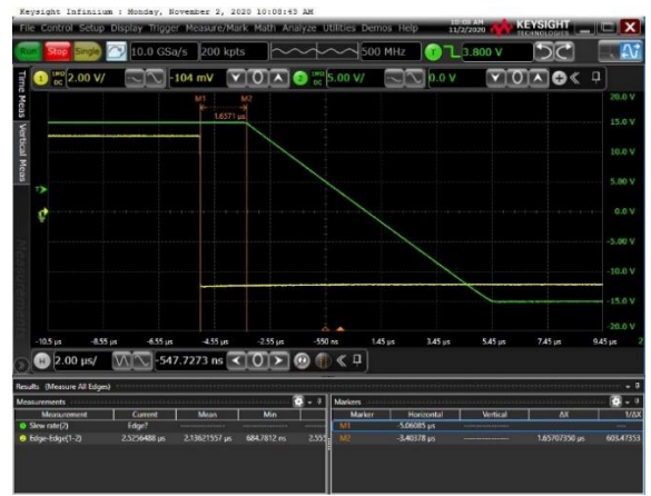
Voltage: 5V/div for Output, Time: 2us/div G=10, VREF = GND; VIN=10VPP, Load R=10K C=100pF
