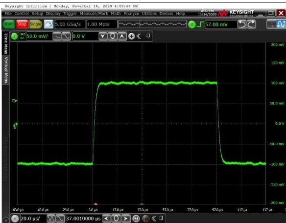
Voltage: 50mV/div for Output, Time: 20us/div G=100, VREF = GND; VIN=2mVPP, Load R=10K C=100pF Figure 29 Small-Signal Pulse Response
