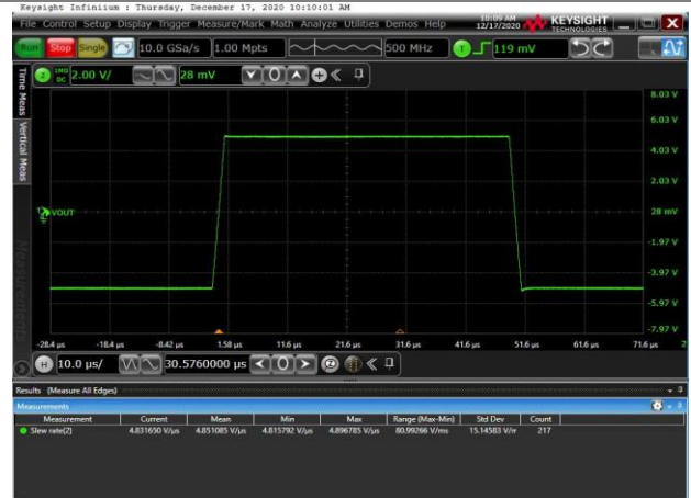
Voltage: 2V/div for Output, Time: 10us/div G=1, VREF = GND; VIN=10VPP, Load R=10K
