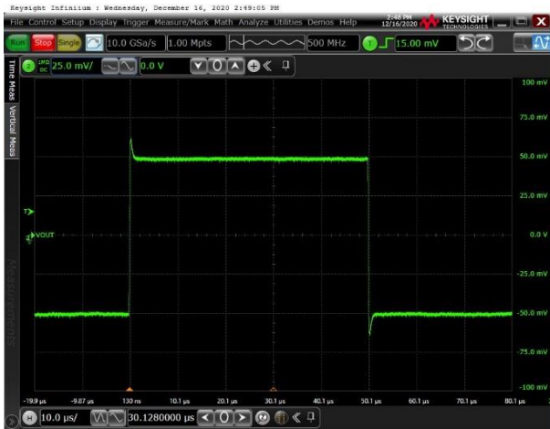
Voltage: 25mV/div for Output, Time: 10us/div G=1, VREF = GND; VIN=100mVPP, Load R=10K C=100pF Figure 27 Small-Signal Pulse Response
