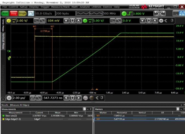
Voltage: 5V/div for Output, Time: 2us/div G=10, VREF = GND; VIN=10VPP, Load R=10K C=100pF
