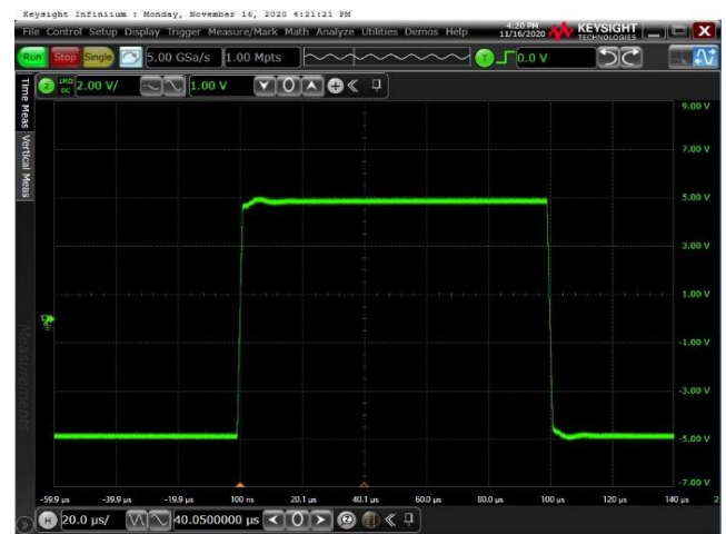
Voltage: 2V/div for Output, Time: 20us/div G=10, VREF = GND; VIN=1VPP, Load R=10K C=100pF
