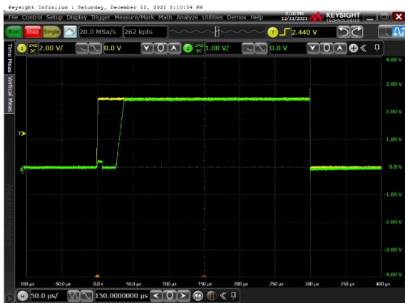
Figure 25. Power On and Off Behavior, G = 1 , V_{IN} = 0.5\text{ V} during Power On and Off, Yellow: +V_S , Green: Output
