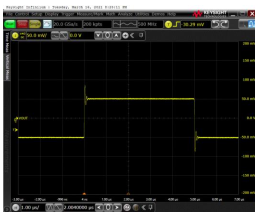
Figure 17 Small Signal Step Response
