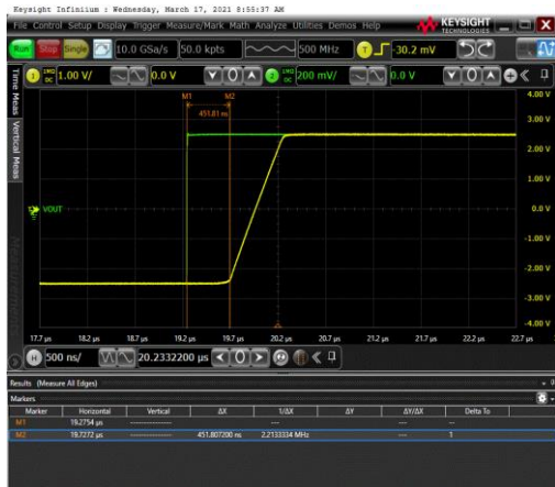
Figure 15 Overload Recovery at Negative Rail
