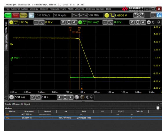
Figure 16 Overload Recovery at Positive Rail
