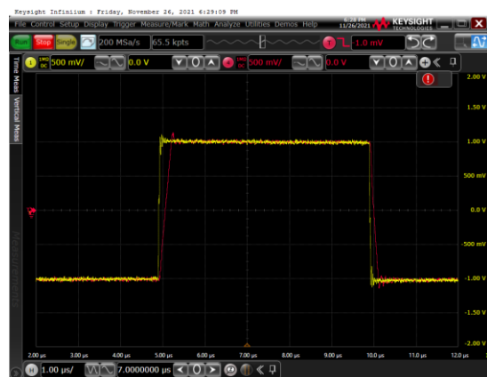
Figure 18 Large Signal Step Response
