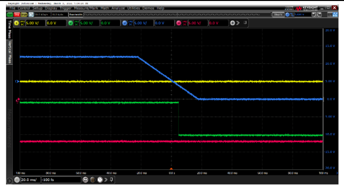
Blue >>AVCC, Yellow >>VDD, Red >>AVSS, Green >>DAC OUTPUT Code 0xFFF, DAC range: -10 to 0 V, no load Figure 20. DAC Output With AVCC Supply Collapse
