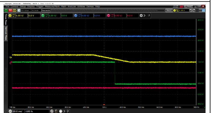
Blue >>AVCC, Yellow >>IOVDD, Red >>AVSS, Green >>DAC OUTPUT
