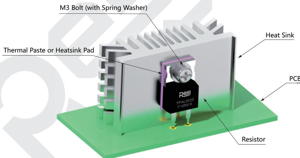
(1) The general installation of TO220 resistors is shown in the figure above. For good thermal conductivity, thermal paste or heatsink pads must be used at the contact position between the bottom of the resistor flange and the heat sink, to ensure contact area for heat dissipation.
