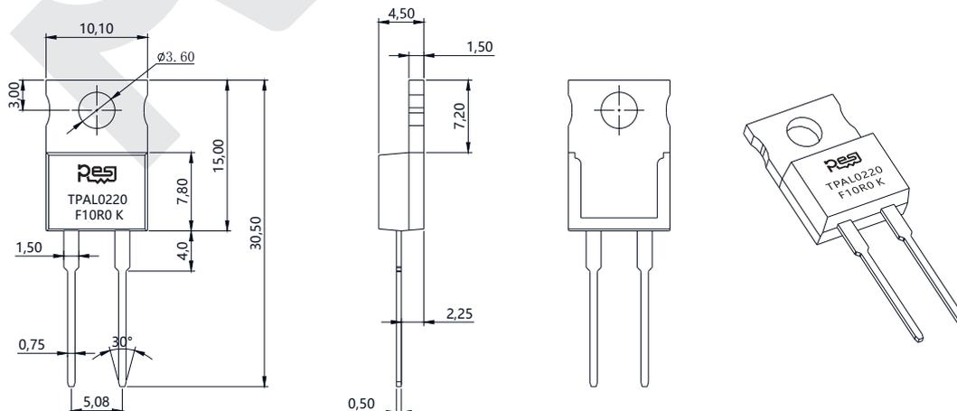
Note: The above dimensional tolerance is ± 0.3mm.
