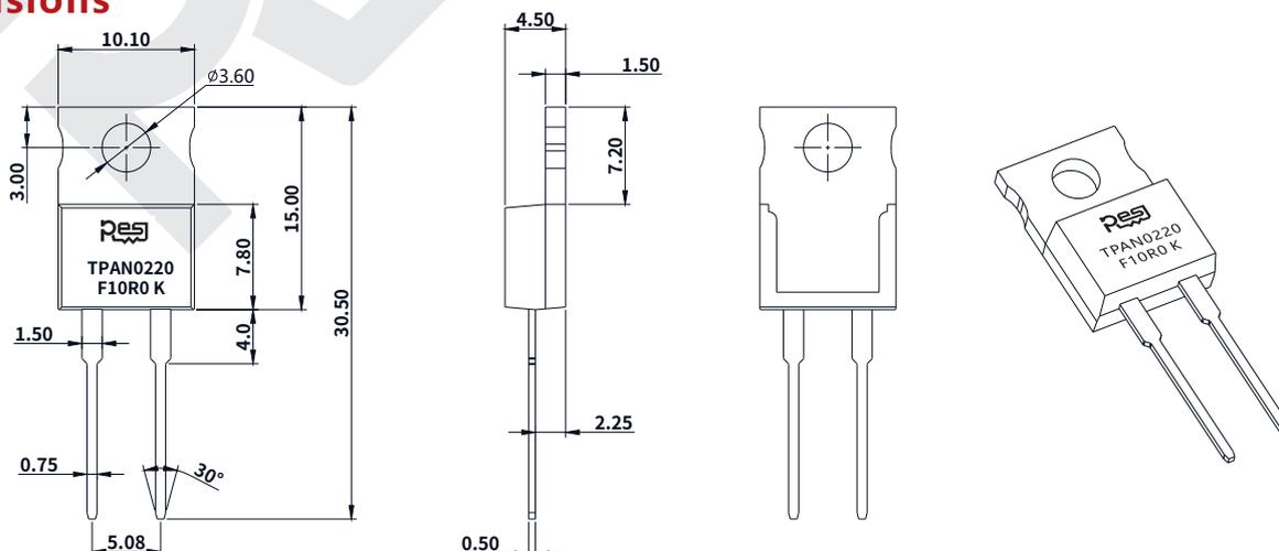
Note: The above dimensional tolerance is ±0.3mm.
