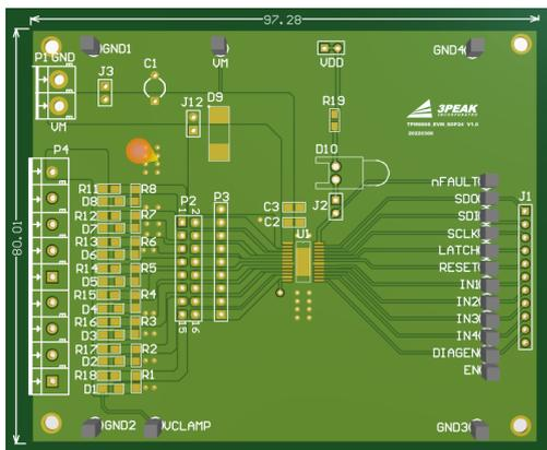
**48-V 8-Ch Smart Low-side Driver Array with Diagnostics and CRC**
