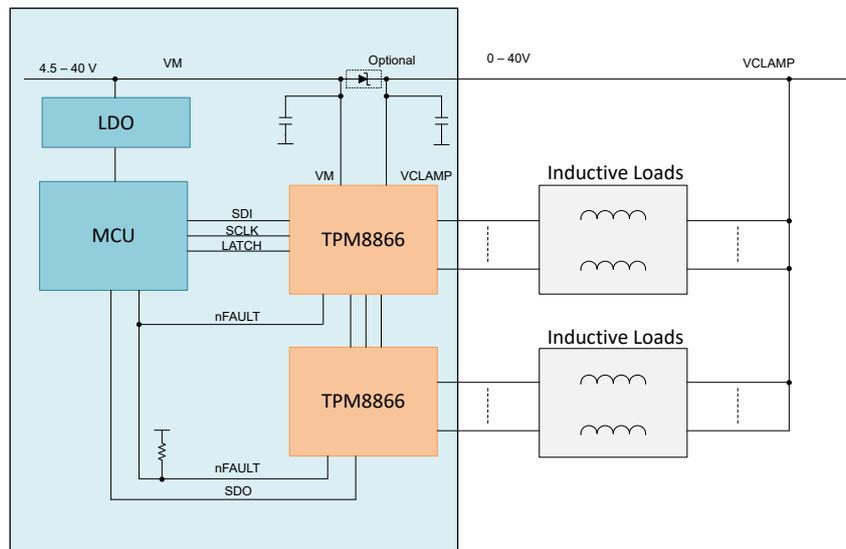
Figure 20. Typical Application Circuit
