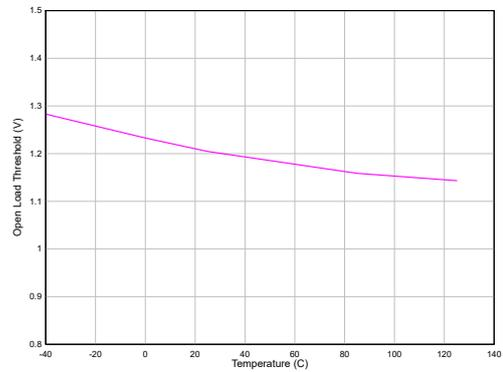
Figure 8. Open-Load Protection Threshold vs. Temperature
