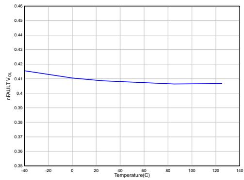
Figure 4. nFAULT  $V_{OL}$  vs. Temperature
