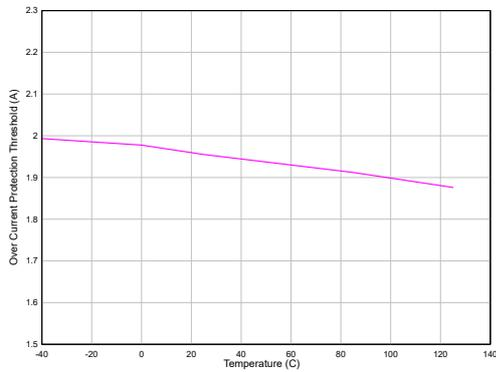
Figure 7. Over Current Protection Threshold vs. Temperature
