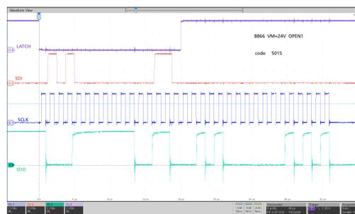
**Figure 19. Serial Communication Read**
