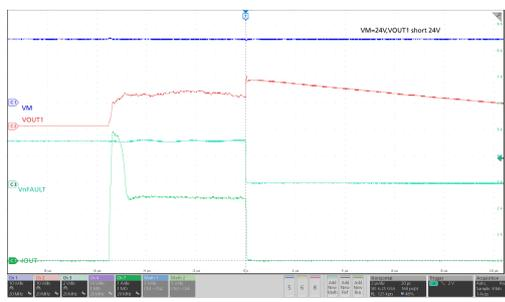
Figure 13. Short Circuit Protection
