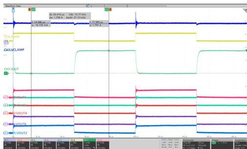
Figure 9. Inductive Load Driving
