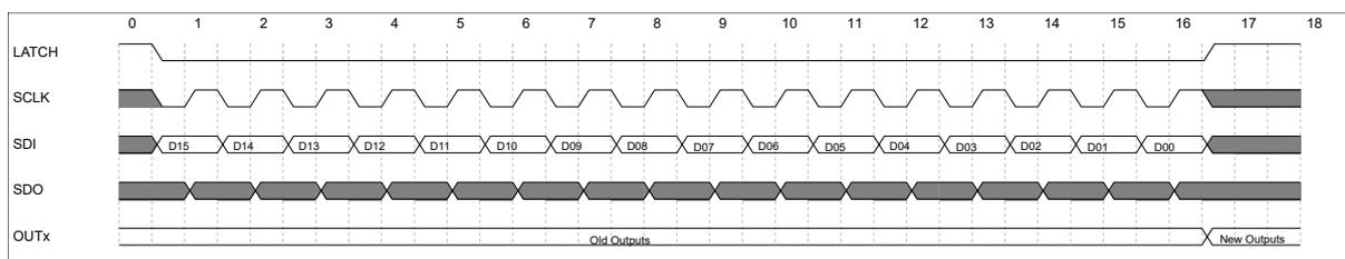
During a read operation, the microcontroller should first issue a write command with the address, and then send out the serial clock when the device selection is high. On each falling edge of SCLK, the device shifts out the data from the internal register to SDO.
