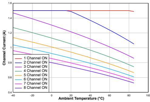
Figure 15. Output Current Capability
