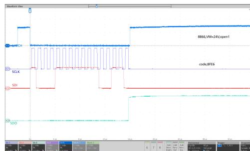
**Figure 18. Serial Communication Write**
