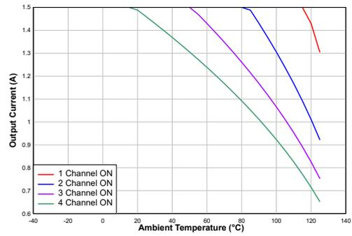
Figure 16. Output Current Capability - Parallel Mode
