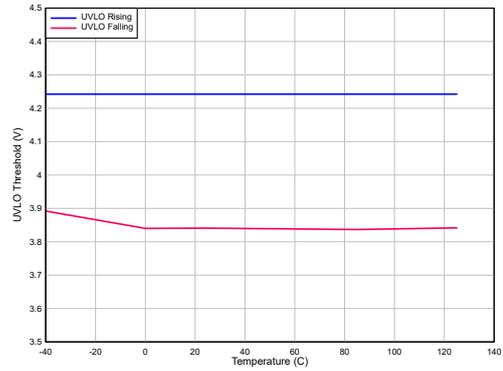
Figure 2. UVLO Threshold vs. Temperature
