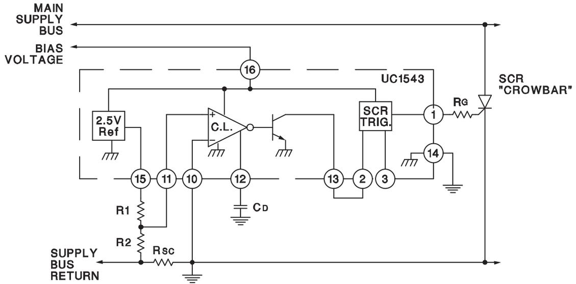
Figure 10. Overcurrent Shutdown
