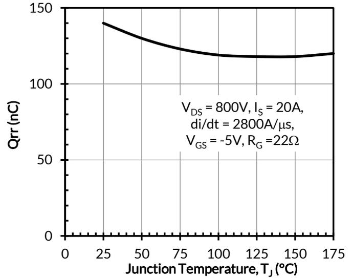
Figure 22. Reverse recovery charge  $Q_{rr}$  vs. junction temperature
