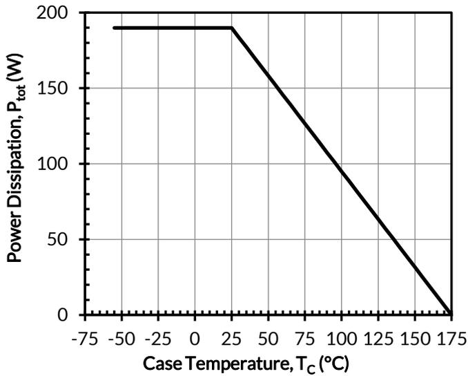
Figure 15. Total power dissipation
