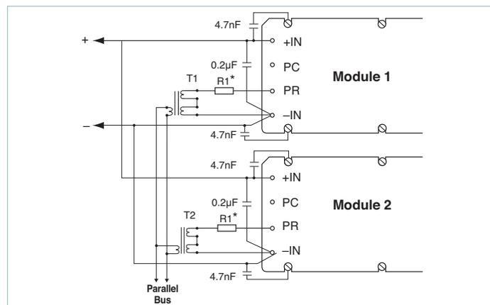
Figure 10 — Transformer-coupled interface
