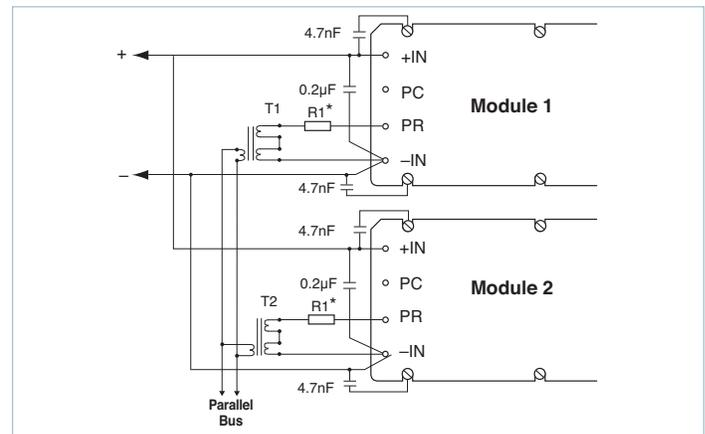
Figure 10 — Transformer-coupled interface
