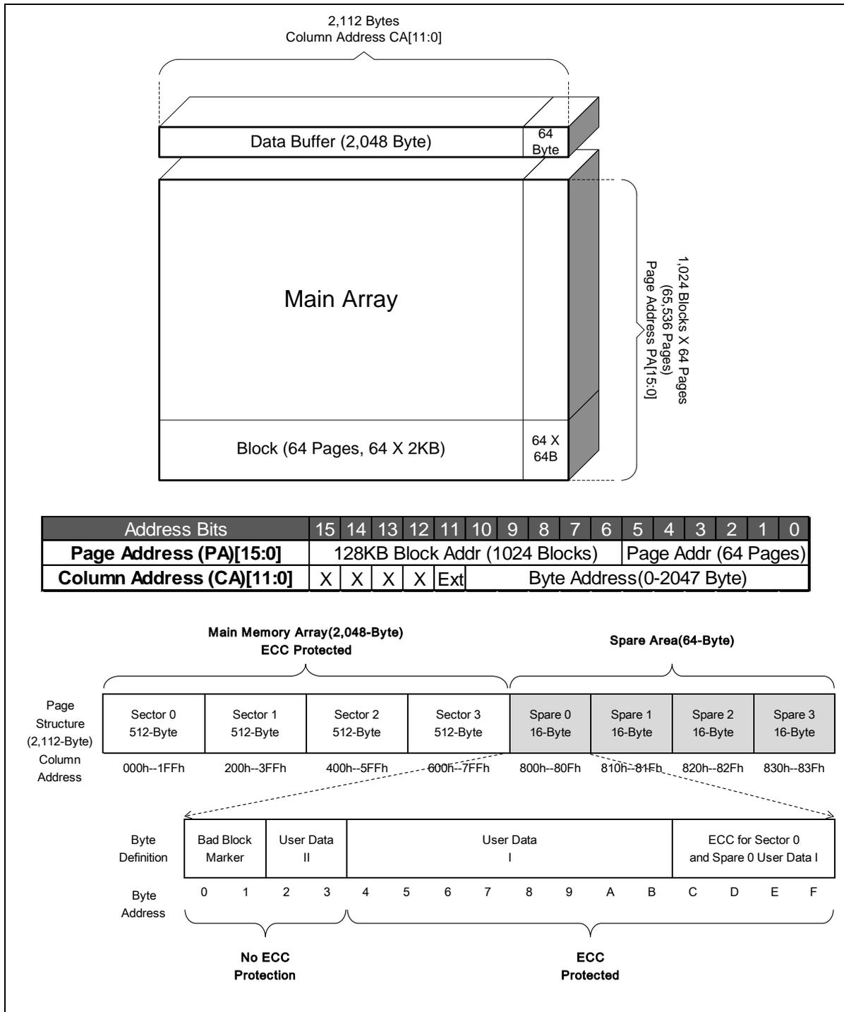
Figure 5-1 W25N01JW Flash Memory Architecture and Addressing
