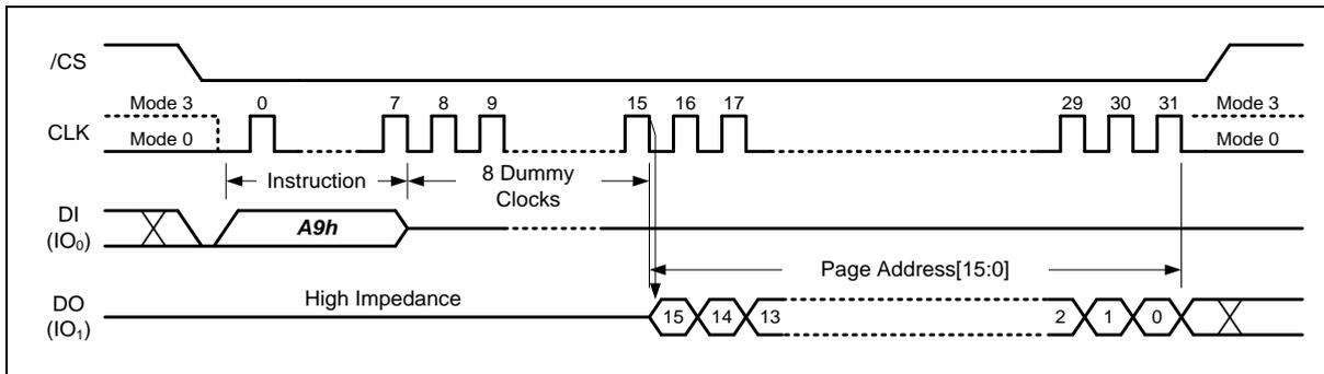
Figure 8-11 Last ECC Failure Page Address Instruction
