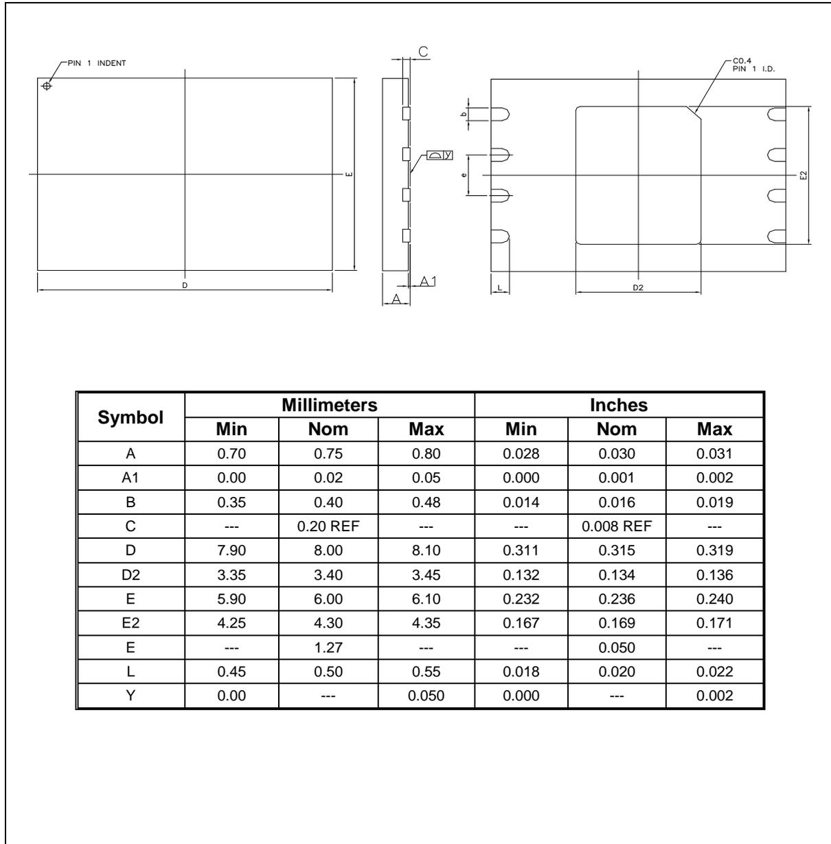
Figure 11-1 8-Pad WSON 8x6-mm (Package Code ZE)
