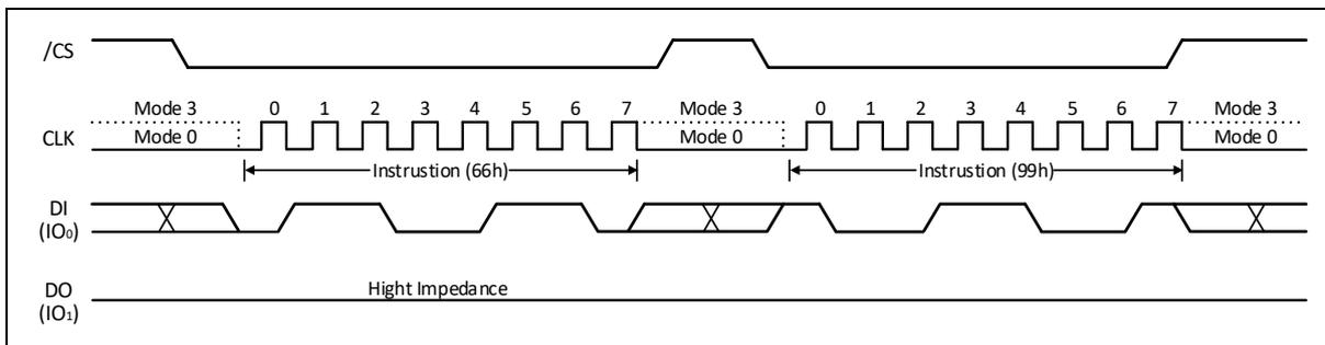
Figure 8-2 Device Reset Instruction (66h+99h)
