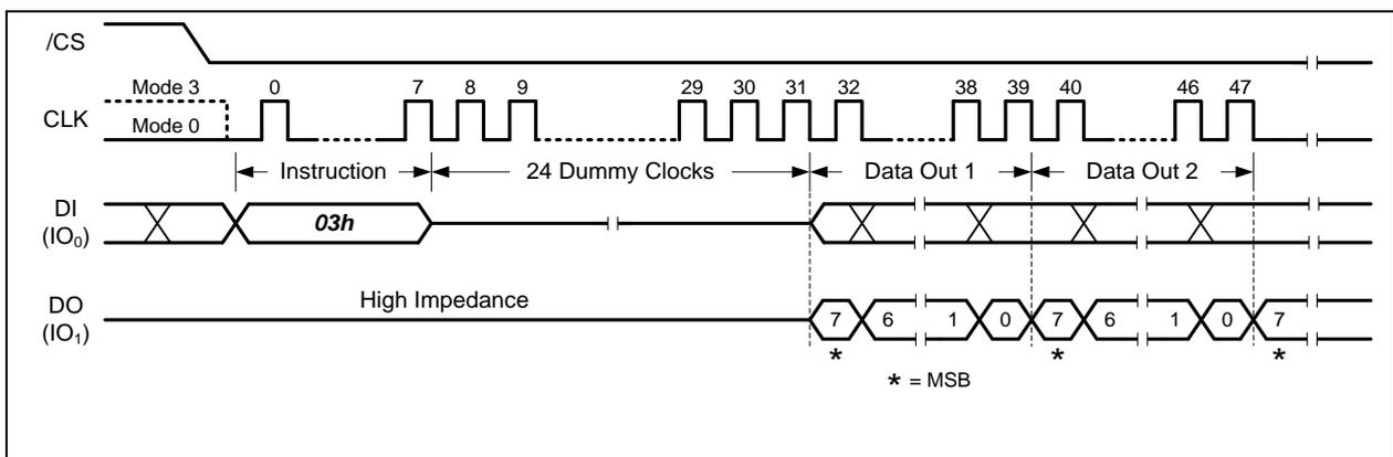
Figure 8-20 Read Data Instruction (Continuous Read Mode, BUF=0)
