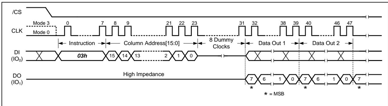
Figure 8-19 Read Data Instruction (Buffer Read Mode, BUF=1)
