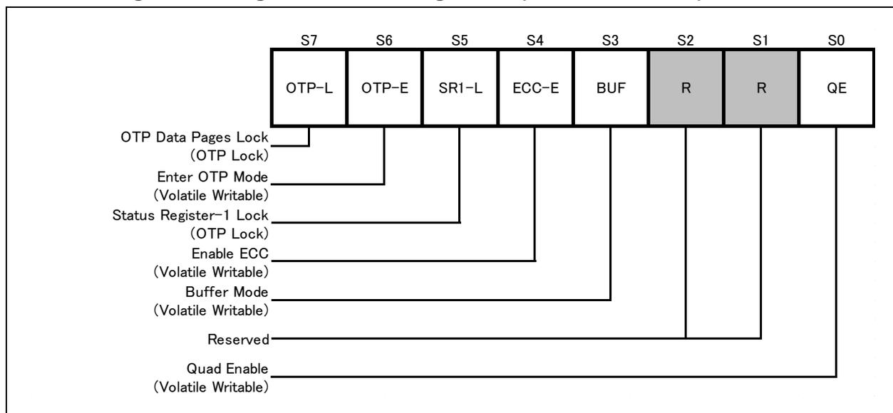
Figure 7-2 Configuration Register / Status Register-2 (Address Bxh)
