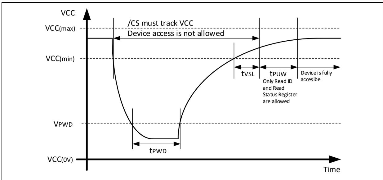
Figure 9-1 Power-up Power-down Timing and Voltage Levels
