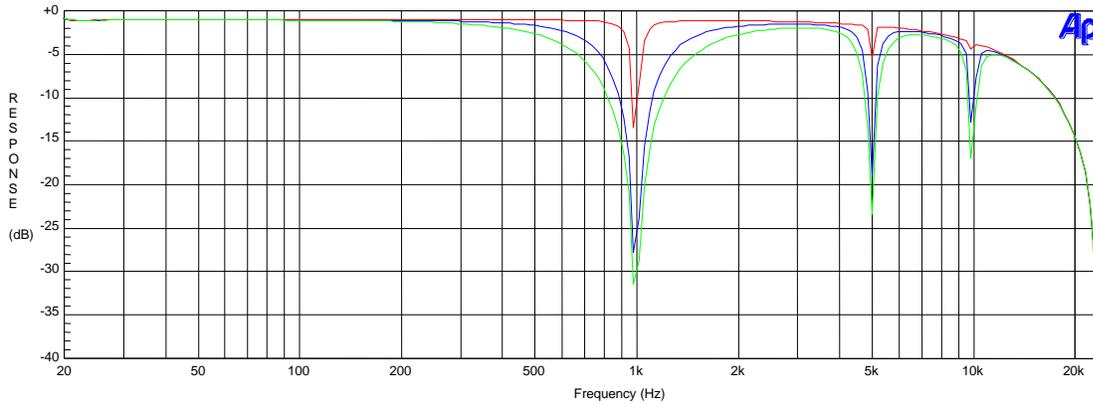
**Figure 48 Cumulative Notch + Low Pass Filters Responses (48kHz);**
