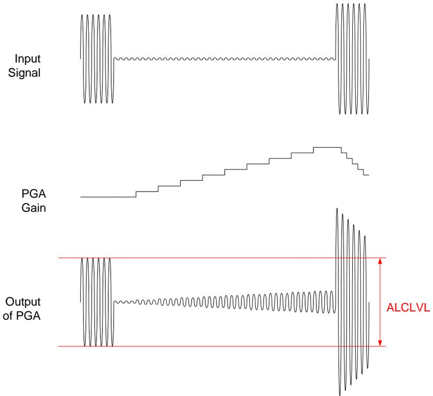
**Figure 17 ALC Operation Above Noise Gate Threshold**
