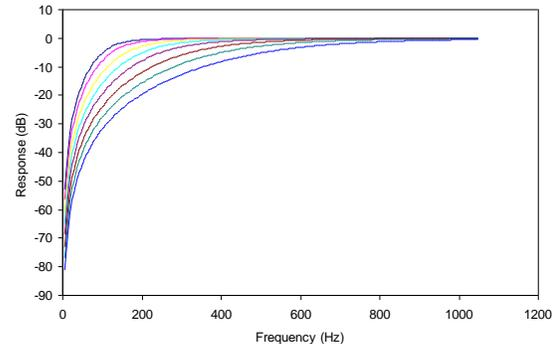
**Figure 45** ADC Highpass Filter Responses (12kHz), HPFAPP=1, all cutoff settings shown.
