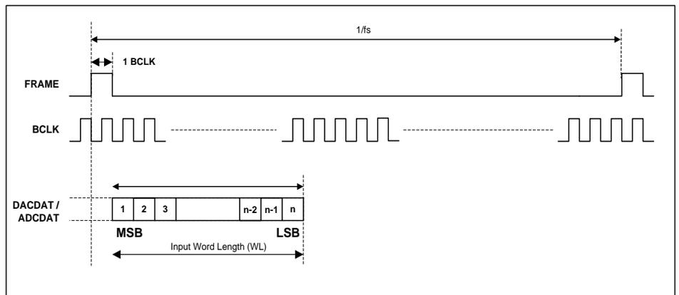
**Figure 28 DSP/PCM Mode Audio Interface (Mode A, FRAMEP=0)**
