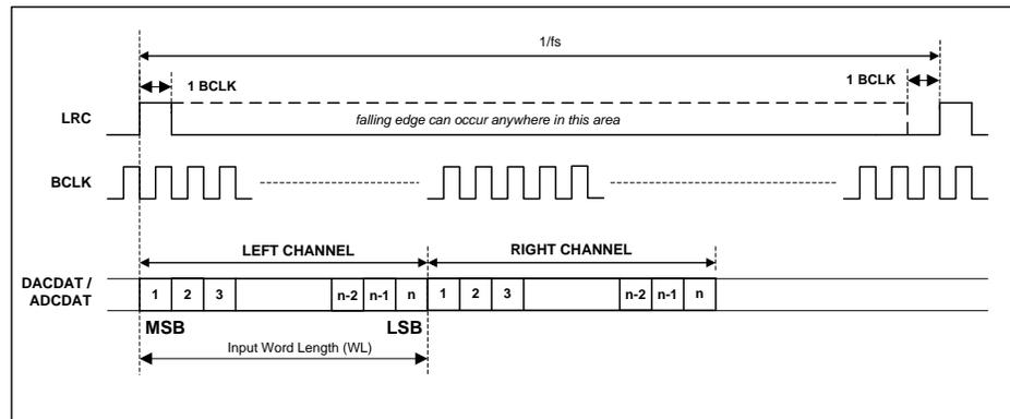
**Figure 29 DSP/PCM Mode Audio Interface (Mode B, FRAMEP=1)**
