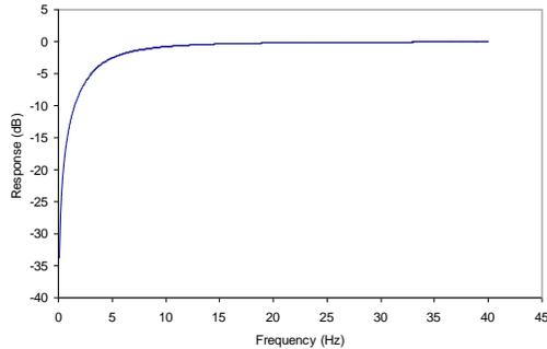
**Figure 42** ADC High pass Filter Response, HPFAPP=0
