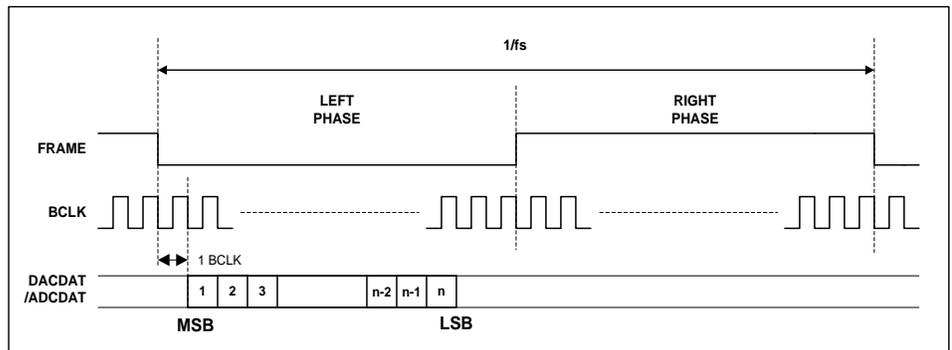
**Figure 27 I<sup>2</sup>S Audio Interface (assuming n-bit word length)**
